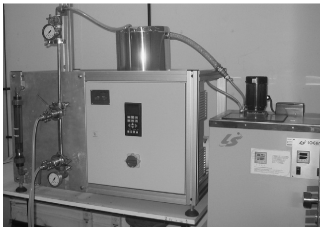
Fig. 1. Experimental ultrafiltration unit.
